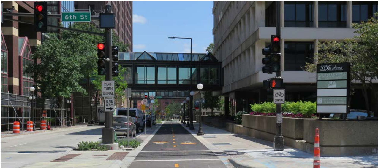
Bicycle signal lens with supplemental plaque. Note the right turn signal with a blank out sign to restrict turns across the bikeway during the bicycle signal phase. Jackson Street, Saint Paul, MN
