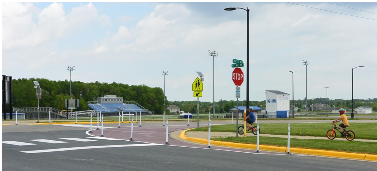
Image 4.06: Children on bikes preparing to cross the street at a curb extension
